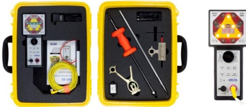
**SNT-02 kit (above) includes the SNT instrument, ground rod with slide hammer, clamps and other accessories.** Go to [www.stepandtouch.com](http://www.stepandtouch.com) for more information.
